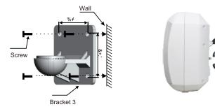
3. According to the installation plan in the adjustable range, adjust the most appropriate height, and then tighten the screws.
