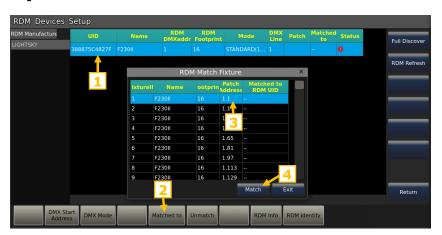
Note: The device should be set to the same channel mode as the patched fixture and it can only be matched to the fixture that is patched in the same DMX line.
