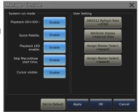
**Quick Palette** --- The option defaults to **[Enable]**. You can recall presets without selecting fixtures. If the option in **[Disable]**, you have to select the fixtures before recalling presets. If you do not select any, the presets cannot be recalled.
