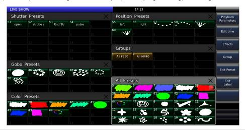
Note: Save the preset in its type of 'Presets' window, the data will be updated to the 'All Presets' window automatically. However, the presets saved in the 'All Presets' window will not be updated to any individual type of 'Presets' window.
