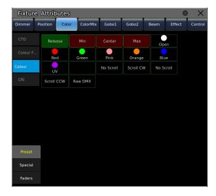
• The **[Special]** option provides a more convenient method for some channels that can mix control. For example, set Pan and Tilt in Position, mix RGB or CMY colors in Color-Mix, or shape cut in Beam.
