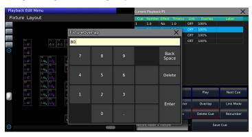
The running time will be divided equally for each fixture. That means if there are 5 fixtures run in 10s for the step. After setting the fixture overlap, each fixture uses 2s to finish its effect.
