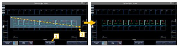
• When **[Step Increment=1]**, the sequence number of the fixtures selected by drawing a selection box increase 1 automatically. The sequence number increases according to the drawing way of the selection box,
