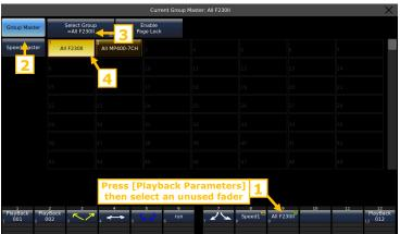
When playing a playback that includes the fixtures in this group, the intensity output value is based on the saved values and the position of the master and Group-Master fader.
