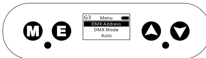
The top left corner of the menu will display the abbreviation of the current wireless protocol mode, which is G3, GZ, and WI.
