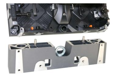
3. To unlock the vertical connector, press the spring-loaded locking latch inward. The vertical connector will then drop open.
