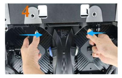
3. Twist vertical connector the left & right to lock.
