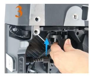
4. Push the locking bar up into locking latch.
