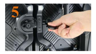
To unlock, rotate handle clockwise, releasing the tension of the horizontal tab- keyed connector cinching mechanism.
