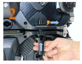
• The spring-loaded locking latch will toward the left then pressing the vertical connector upwards into the locking latch.
