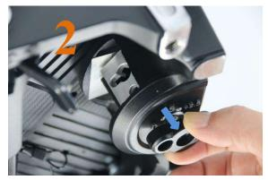
• Lift the arc lock handle and rotate it to the desired angle mark.
