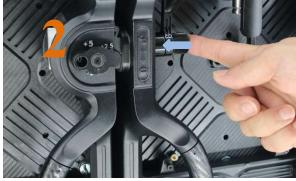
Press the horizontal tab-keyed connector until the tab-key passes through the tab-keyed socket.
