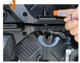
• To unlock, twist the vertical connector level to the right while pressing the spring-loaded locking latch toward the lift.
