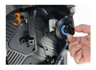
• Release the handle and the arc lock will automatically secure the angle.
