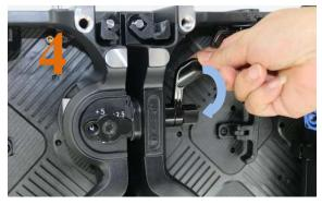
Rotate handle downward (counterclockwise) to cinch the horizontal tabkeyed connector.
