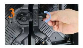
• Rotate the handle to the right (clock- wise) to hold the horizontal tab-keyed connector in place.
